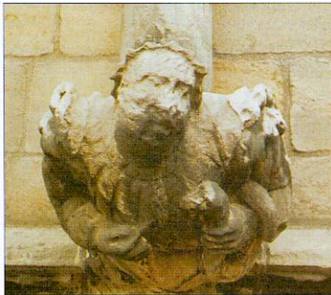
FIGURE 9.27 Atmospheric acids, especially sulfuric and nitric acids, have almost completely eaten away the face of this medieval statue. Each year, the total losses from air pollution damage to buildings and materials amount to billions of dollars.
